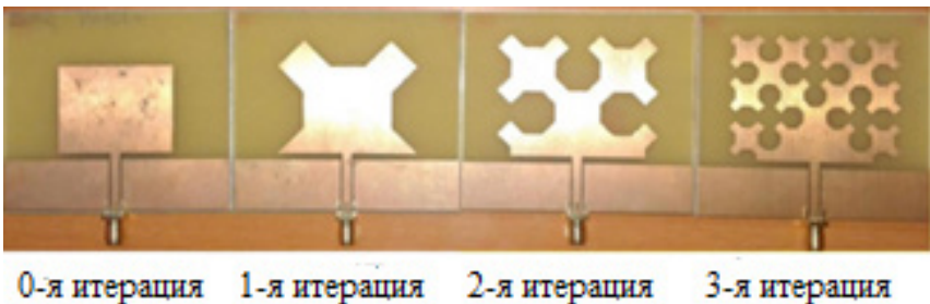
Figure 2 – Fractal antenna "Sierpinski cross" [2]
